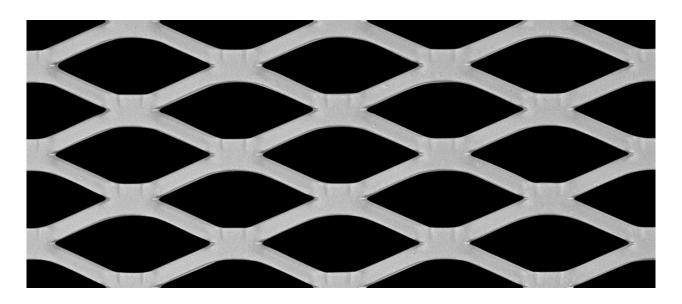
LW Aperture:42.93mmStrand Width:4.60mmSW Aperture:14.22mmThickness:2.69mmWeight:8.59 kg / m2Open Area:61%
